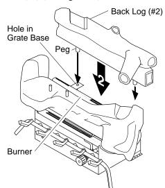
Figure 22 - Installing Back Log (#2)
